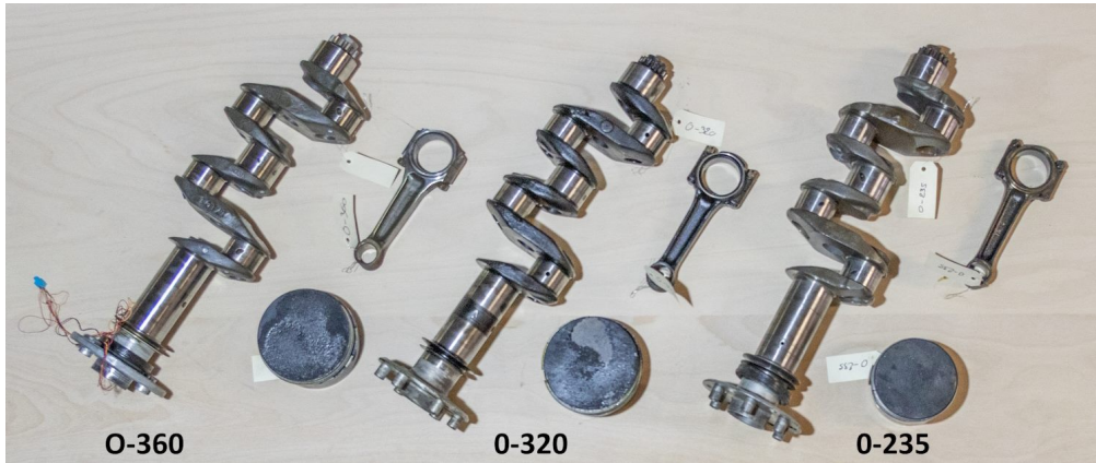
Lycoming crankshaft assemblies (O-360, O-320, O-235) instrumented with internal strain gauges for torque measurement
