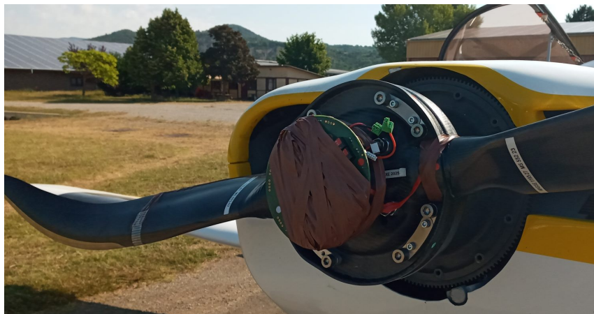
ELIAS electronic board integrated into an instrumented propeller hub
