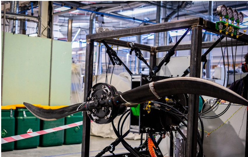
RESONATOR test bench --- a propeller under torsional vibratory load
