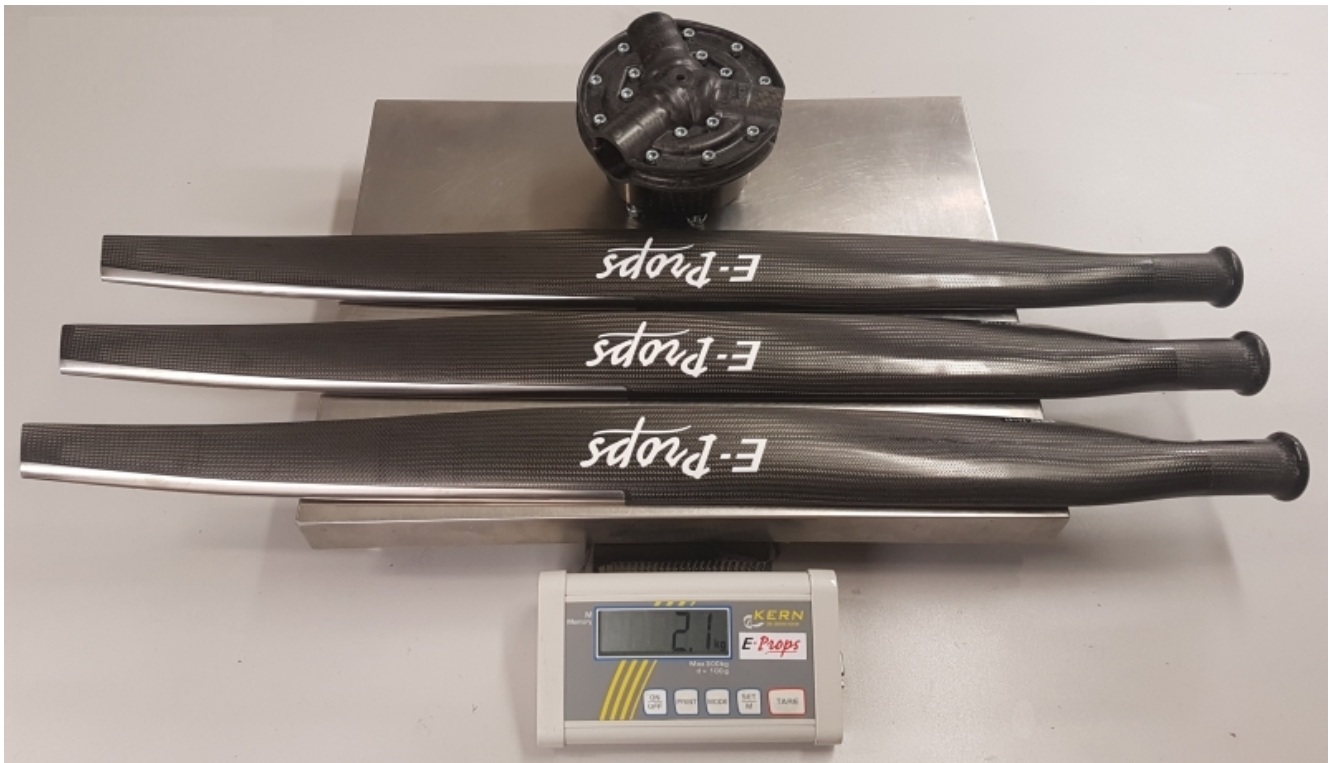
3-blade ground adjustable model diameter 170 cm, Titanium leading edge protection, with all screws = 2,1 kg
