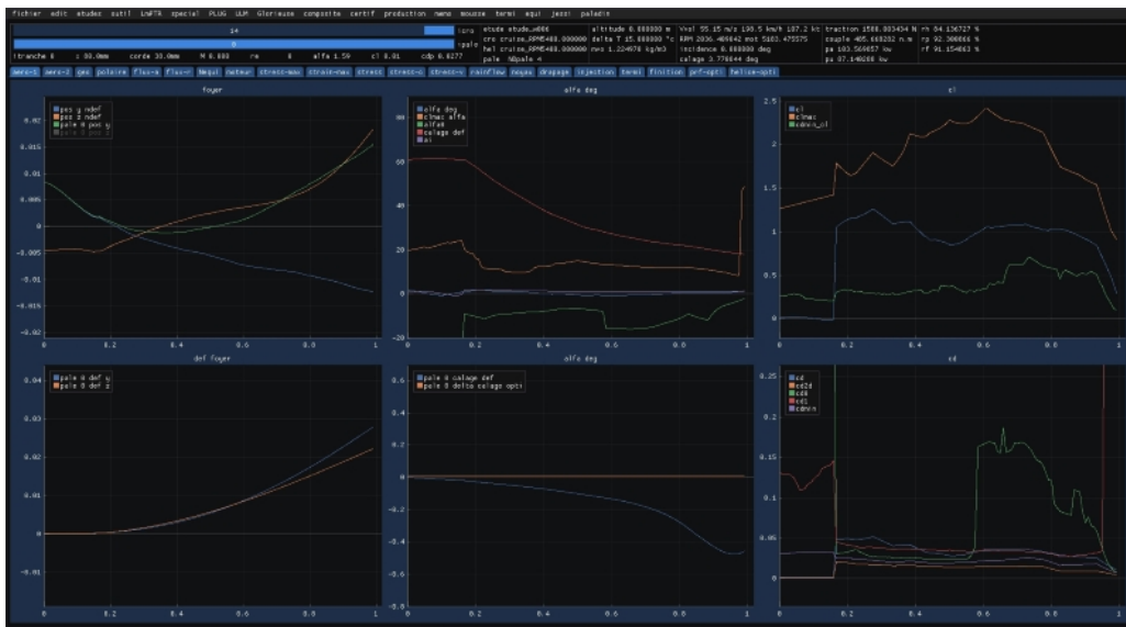
LUKY --- evolution of a candidate blade's local aerodynamic parameters (angle of attack, pitch, lift and drag coefficients) along the span, during optimization
